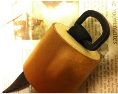
Figure 10. Piston with shock cord attached
