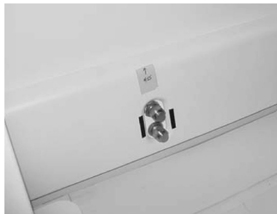
Figure 14. Multi-User Overboard Vent
