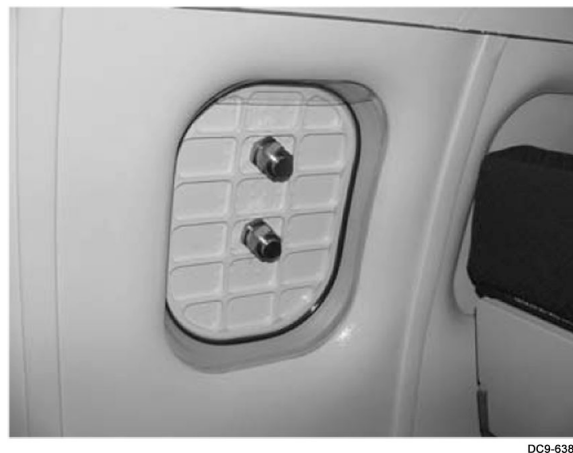
Figure 15. Dedicated Overboard Vent Ports
