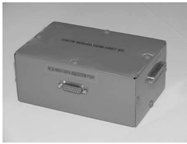
Figure 16. Signal Distribution Box
